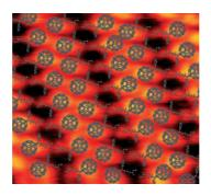
Controlled hydrogen bonding: At high coverage, the self-assembly of a fullerene derivative (PCBM) on the Au(111) surface (see figure) is primarily controlled by hydrogen bonding between the PCBM tails. Gas phase simulations agree well with experiments, as due to the large size of the fullerene cage, the hydrogen bonds are far away from the surface.
